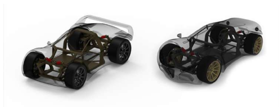
Figure 32. Car bodies showing the shared Chassis.
