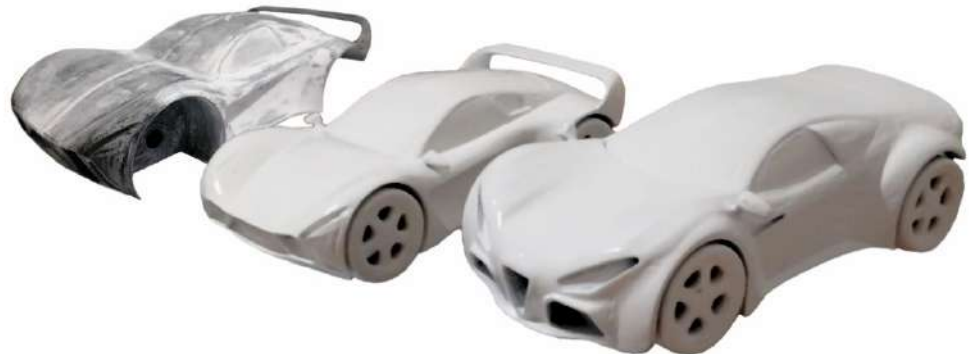
Figure 37. Mockup model in the post-process phase (left) and completed mockup models (right).
