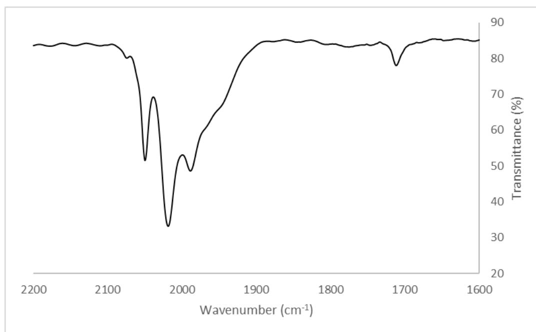
Figure S3. IR spectrum in the \nu_{\text{CO}} region of [\text{NEt}_4][\text{AuRu}_5(\text{CO})_{19}] ( 4 ) in \text{CH}_2\text{Cl}_2 .
