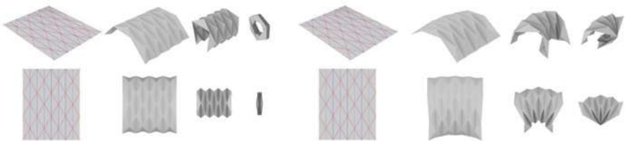
Figure 87 - Folding physical simulation of a traditional “Yoshimura” origami pattern, with uniform and non-uniform fold angle distribution.
