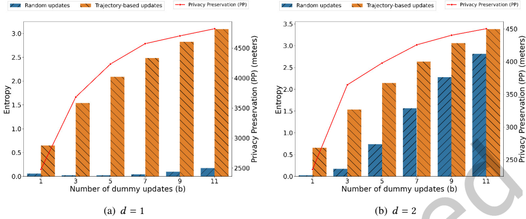
Fig. 9. The entropy and PP metrics as a function of the number of dummy updates in a random Dummy Updates scheme and a trajectory-based one.
