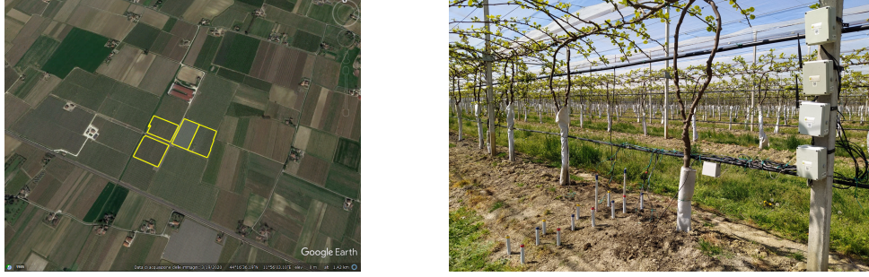
Figure 4: A sensor grid is monitoring soil moisture close to a kiwi tree near Faenza, Italy. The watering system is composed of single-pipeline drippers.
