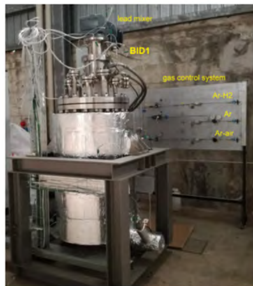
Figure 29. BID1 pool facility, equipped with lead mixer and gas control system based on H 2 and air injection.
