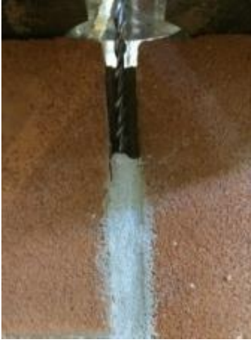
Failure mode B: bar pull-out
