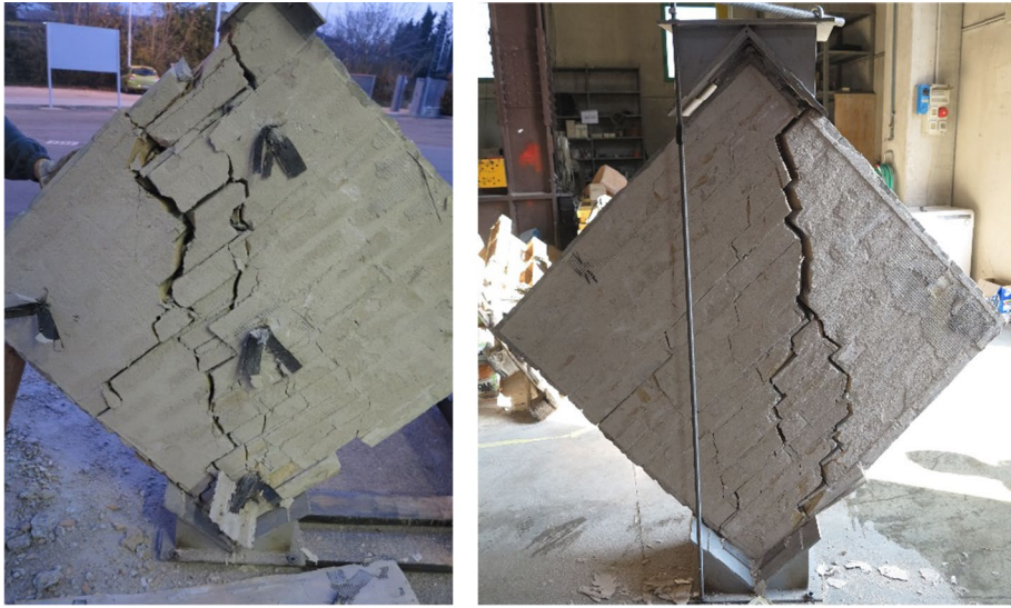
Fig. 11 Diagonal compression test: failure mode of the FRCM strengthened samples
