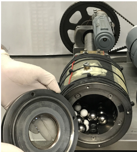
Fig. 2a and 2b. The ball mill. a) the ball mill machine used in this study just after spheres loading; b) rubber-lined steel racks with specimens already positioned in their receptacles.
