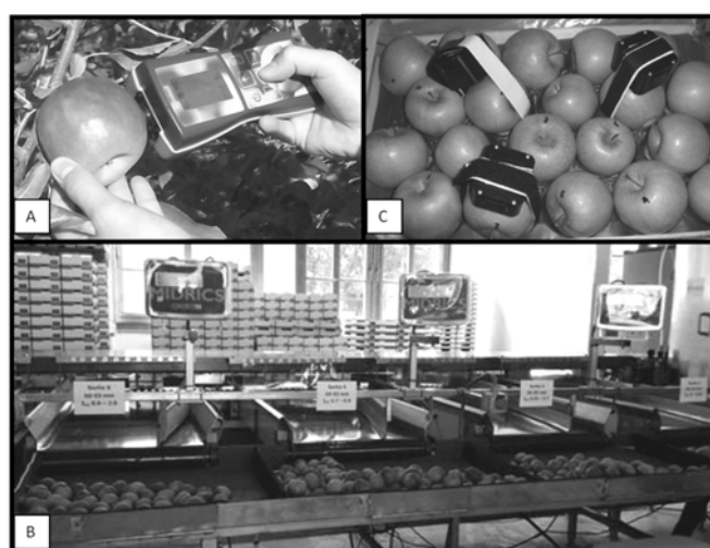
Figure 1. The three devices assessing fruit ripening ( I_{AD} ): (A) the DA-Meter at field level; (B) the DA-Head at the packinghouse level; and (C) the DAFL in cold storage.
