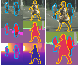
Figure 4. The rightmost column is synthesized by copying pixels from the left column into the central one. Pixels are chosen according to their semantic class (second row) and stacked according to their depths (third row). The white pixels in the depth maps represent areas too far from the camera that cannot be selected.
