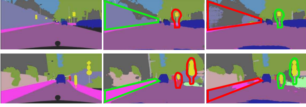
Figure 2. From left to right: ground truth, semantics from depth, semantics by LTIR [22]. The semantic labels predicted from depth are more accurate than those yielded by UDA methods in regularly-shaped objects (such as the wall in the top image and the sidewalk in the bottom one), whilst UDA approaches tend to perform better on small objects (see the traffic signs in both images).
