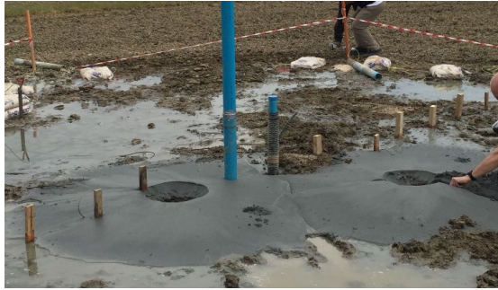
297 298 Fig. 9. Multiple sand boils and ejecta, evidence of liquefaction, observed during blast 1 near the 299 center of the unimproved natural panel (NP).
