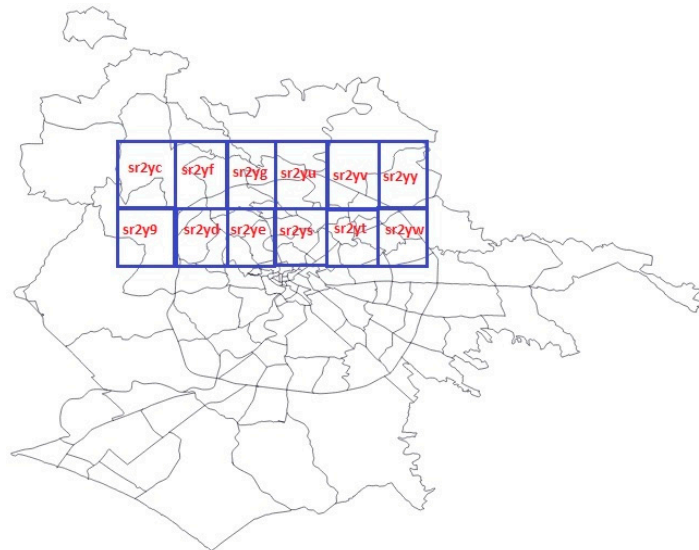
Figure 1. Partial view of the geohash covering near the city center of Rome in Italy. Geohash precision is 25 (i.e., 5 characters). Mobility data traces that are nearby by certain distance are enclosed within the boundaries of the same geohash area; thus, have the same geohash index value. Several geohash values cover a specific neighborhood. This is known as the geohash covering. Edge cases occur in the situation where several points share the same geohash value despite belonging to different neighborhoods. Those cases are resolved by applying the spatial join operator.
