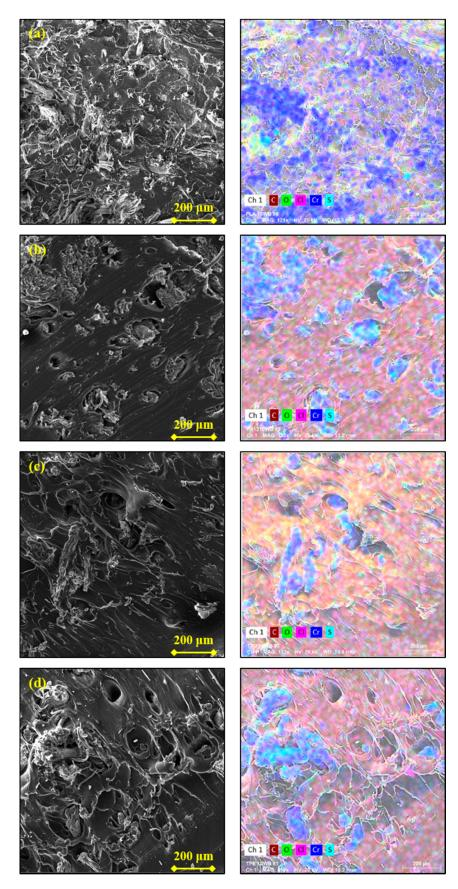
**Figure 6.** Scanning electron microscope (SEM) images of PLA- (**a**), PA12- (**b**), TPU- (**c**), and TPE-based (**d**) composites taken at low magnification (200×) and their corresponding EDS maps on the right.
