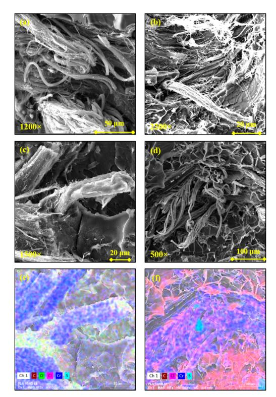
**Figure 7.** Scanning electron microscope (SEM) images of the PLA10WB sample at different magnifications (**a**–**d**); (**e**) EDS map of micrograph (**c**) and (**f**) EDS map of micrograph (**d**).
