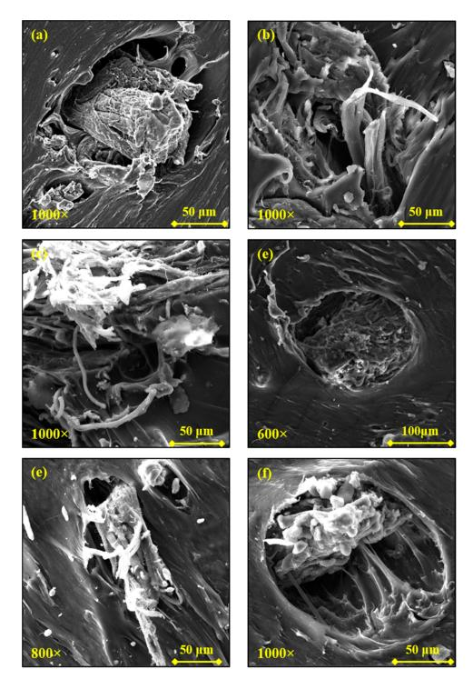
**Figure 8.** Scanning electron microscope (SEM) images of the PA1210WB (**a**,**b**), TPU10WB (**c**,**d**), and TPE10WB (**e**,**f**) samples at different magnifications.
