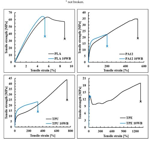
Figure 5. Tensile behavior of WB-based composites.
