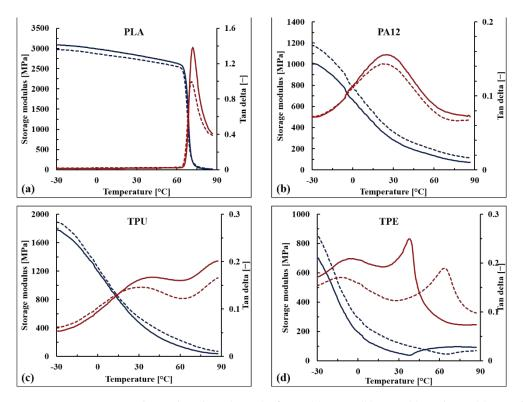
**Figure 10.** Dynamic mechanical analysis (DMA) of PLA (**a**), PA12 (**b**), TPU (**c**), and TPE (**d**) samples. Blue and red curves refer to the storage modulus (E') and the damping factor (tan  $\delta$ ), respectively; meanwhile, the solid and dotted lines indicate the properties of the neat polymer and the corresponding WB-based composite, respectively.
