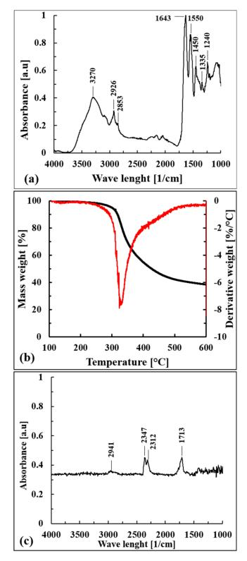
**Figure 2.** (a) ATR spectrum of WB fibers, (b) TGA and DTA curves of dried WB fibers, and (c) FT-IR spectrum of degradative products released by WB fibers at  $T_{peak}$  (328.6 °C).
