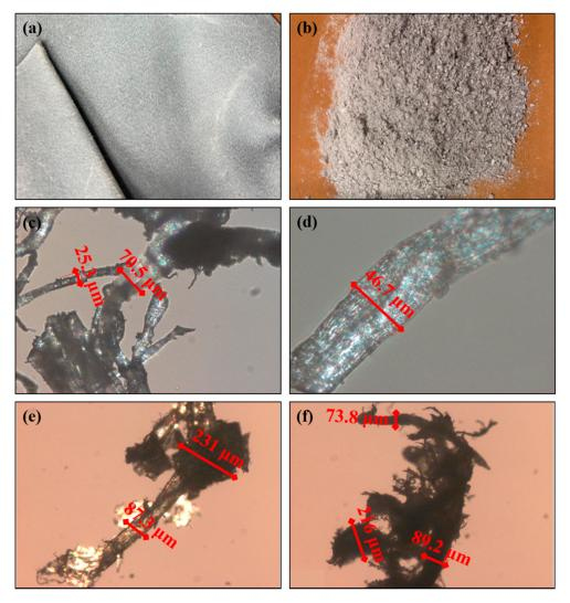
**Figure 1.** Pictures of the WB leather before (**a**) and after (**b**) grinding and images of the grinded WB fibers taken by an optic microscope (**c**–**f**). It is possible to recognize three different structures: the main fibrous body (mean diameter of 70  $\mu$ m), branched and exfoliated tiny fibers (22  $\mu$ m), and bulky and coarse entangled fiber clusters (222  $\mu$ m).
