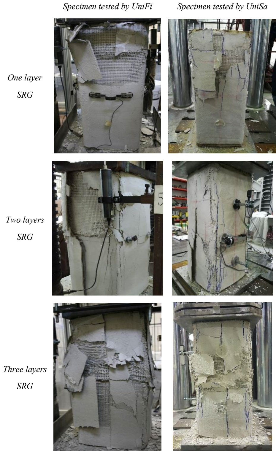
484 Fig. 14. Failure mode of Tuff masonry specimens confined by SRG.
