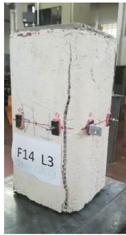
418 Fig. 11. Failure mode of Tuff masonry specimens confined by GFRCM.
