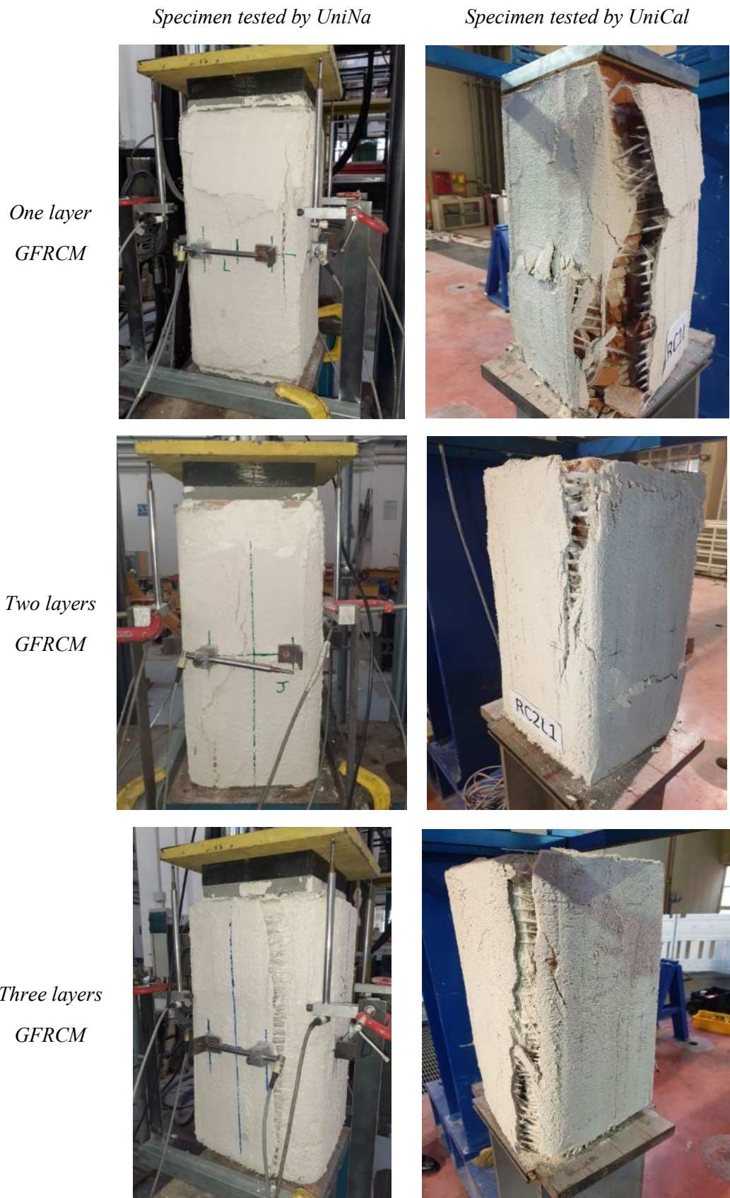
559 Fig. 19. Failure mode of clay masonry specimens confined by GFRCM.
