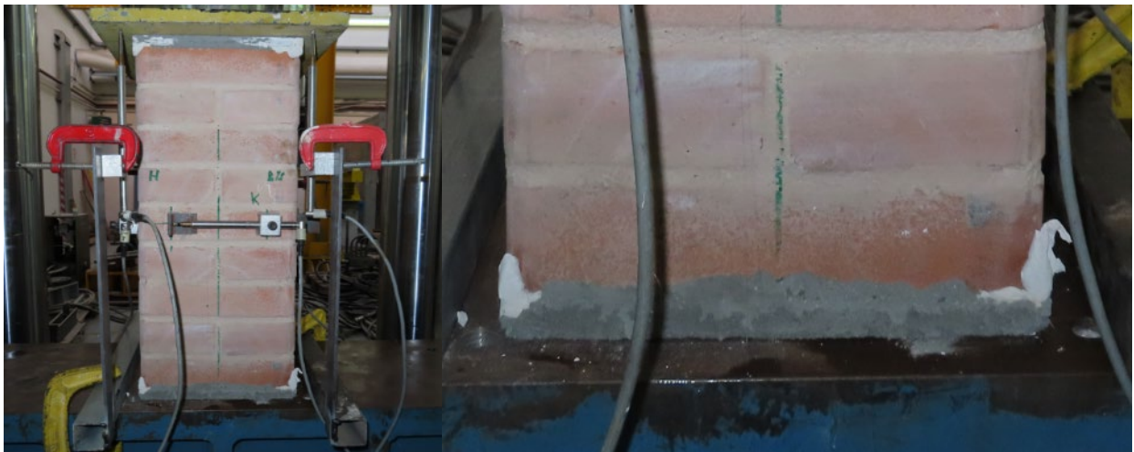
270 271 Fig. 6. Mortar layers placed on top and bottom face of masonry specimens (UniNa).
