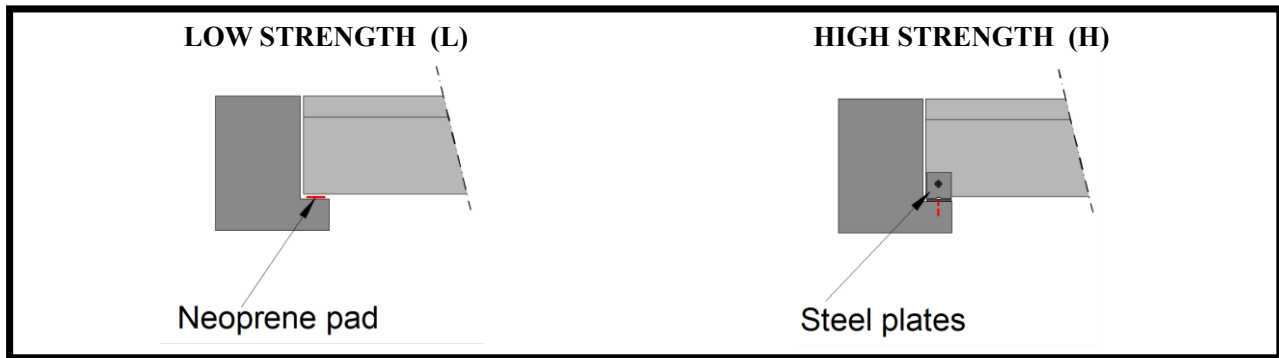
Figure 4. Criteria for the classification of the frame stock.
