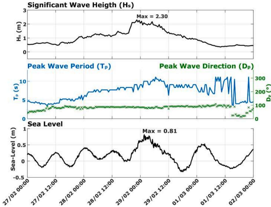
Fig. 2. Measured  $H_s$ ,  $T_p$ ,  $D_p$ , and sea-level during the storm that hit the Emilia-Romagna coast at the end of February/beginning of March of 2016. Wave data was measured every 30 min by a buoy deployed just offshore of Cesenatico (buoy location shown in Fig. 1B). Sea level data was obtained every 10 min by a tide gauge located in the Municipality of Rimini.
