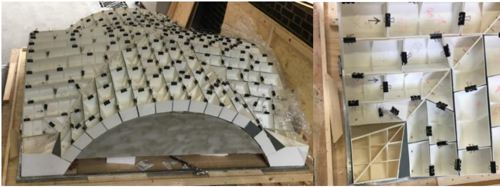
Figure 6: Pre-assembly of the plastic skin of the blocks.
