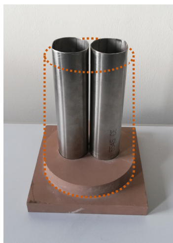
Figure 5. Cylindrical electrodes inserted in the resin base used for the measurement of the electric parameters. The dashed orange lines represent the shape of the PVC tube used to create the container using the resin base as cap.
