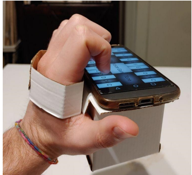
Figure 5. Case prototype. Rear view. This image provides a demonstration of how the handle works.
