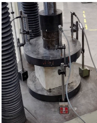
Figure 4. Placement of the three LVDTs on the bottom plate of the testing machine.
