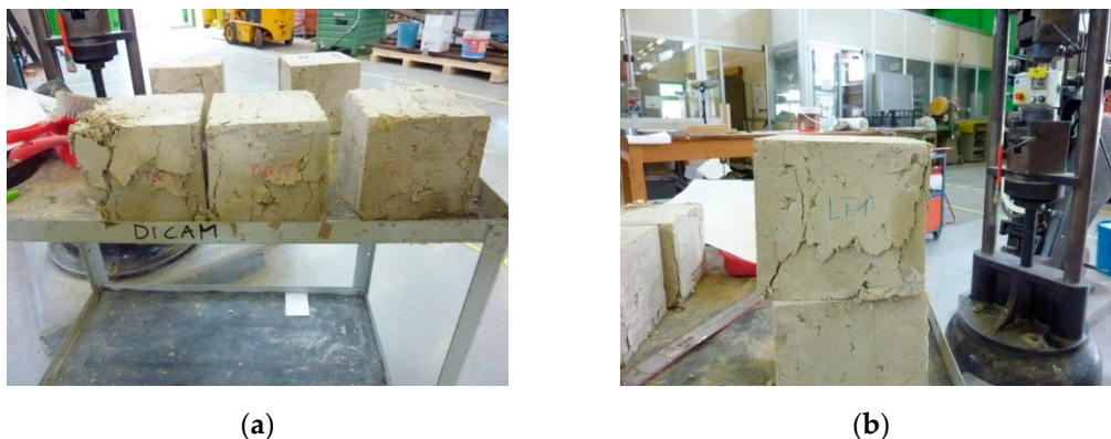
Figure 11. Appearances of the specimens after removal from the testing machine: (a) three TQ specimens in the foreground; and (b) detail of one LT specimen.
