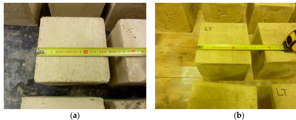
Figure 3. Dimensional checks after drying: (a) TQ specimens; and (b) LT specimens.
