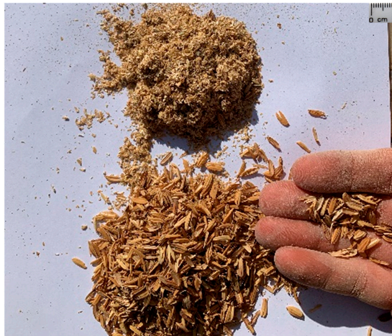
Figure 1. The two types of RH used in the experimental program, arranged by decreasing lengths from bottom to top: unaltered RH (maximum size variable from 6 to 8 mm), and shredded RH (maximum size: 2 mm).
