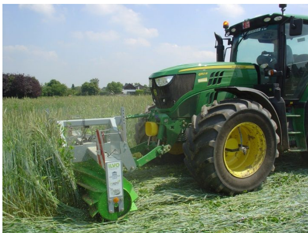
84 85 Picture 3. The roller crimper flattening the ASC in the Research Institute for Agriculture, Fisheries and Food 86 (BE-ILVO) trial.
