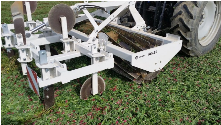
595 596 Picture 188. Machinery used for NT-RC management in the trial established at the University of Maribor (Pivola), 597 Faculty of Agriculture and Life Sciences (UM), Slovenia (SI). A tractor equipped with a roller crimper and in-line 598 tiller.
