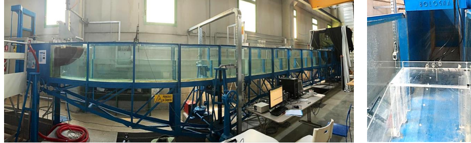
142 143 Figure 1. Wide-angle view of the wave flume (left) and front-view of the structure with crown wall 144 installed at the end of the flume (right).
