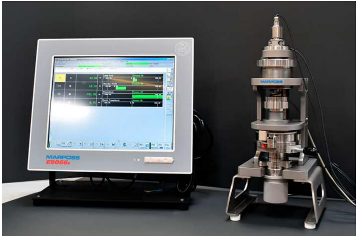
Figure 1. Marposs electrochemical dilatometer with electronic control unit.
