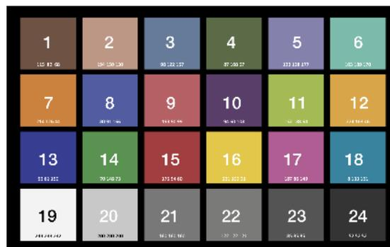
Fig. 5: The target Calibrite ColorChecker Classic.
