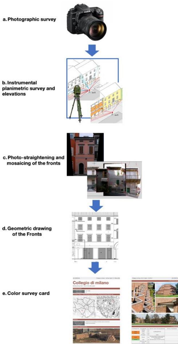
Fig. 1: Imaging workflow from acquisition to the color survey cards.
