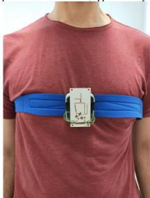
Fig. 7. Photo of the SIL sensor placed at the user's chest for the first set of measurements.
