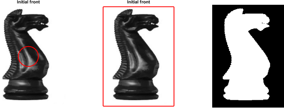
Figure 8: Test 3. From left to right: Initial front for the expansion case (Case 3a) composed by a circle of radius r = 0.5 ; initial front for the shrinking case (Case 3b); mask used for the pixel errors in both cases.
