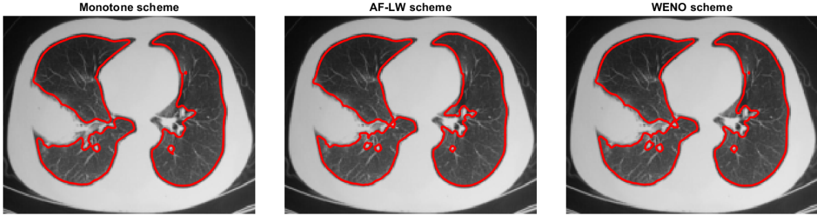
Figure 19: Test 6a with Datum 2. From left to right: Plots of the final front using the monotone scheme ( N_i = 413 ), tol = 0.00001 , the AF-LW scheme ( N_i = 589 ) with tol = 0.00001 , and the WENO scheme ( N_i = 458 ) with tol = 0.000012 , all using L^1 norm, \mu = 4 , K_{reg} = 5 , and velocity \tilde{c} .
