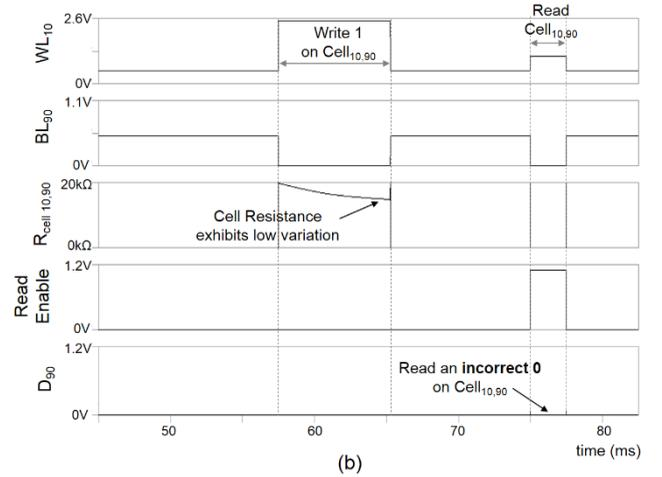
Fig. 3 Simulation results showing the waveforms obtained when first writing a 1, then reading,  $cell_{10,90}$  for: a) a fault free memory array; b) a non-selected  $cell_{10,70}$  with its selector affected by a short, sharing the same wordline  $WL_{10}$  as the selected  $cell_{10,90}$ .
