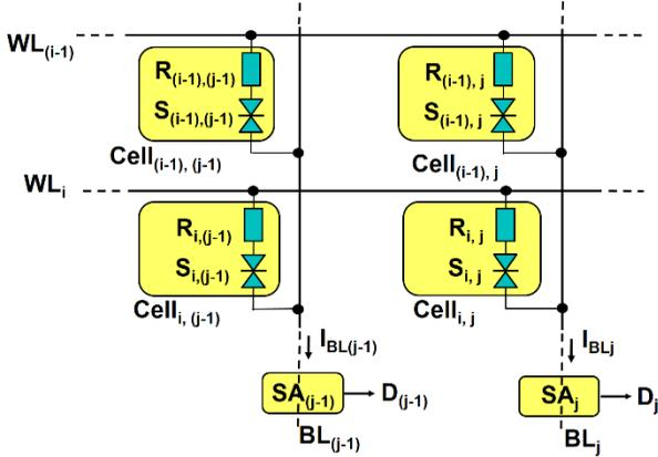
Fig. 1. Schematic representation of a portion of a ReRAM crossbar array.
