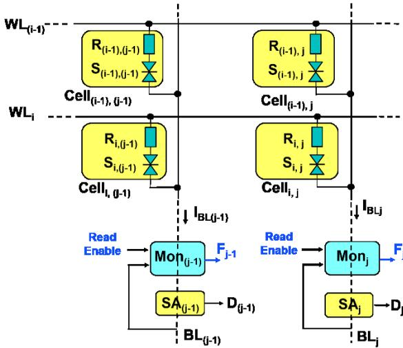
Fig. 5. Schematic representation of our proposed scheme to detect shorts affecting selectors of ReRAMs in crossbar arrays.
