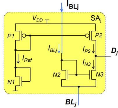
Fig. 2. Schematic representation of the implementation of a current sense amplifier  $SA_j$  of the kind in [13].
