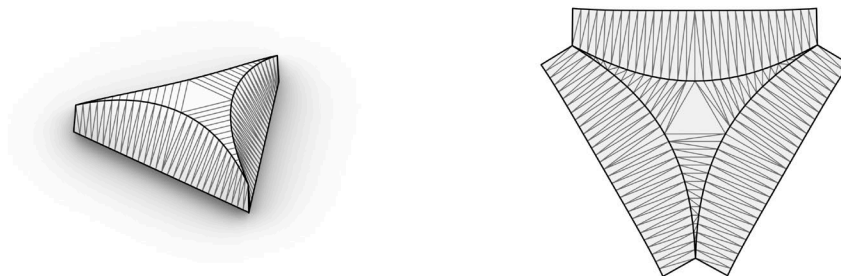
Figure 4: Wrong ruling guessing, which still gives a developable result due to dense triangulation, however the surfaces do not approximate smooth surfaces.
