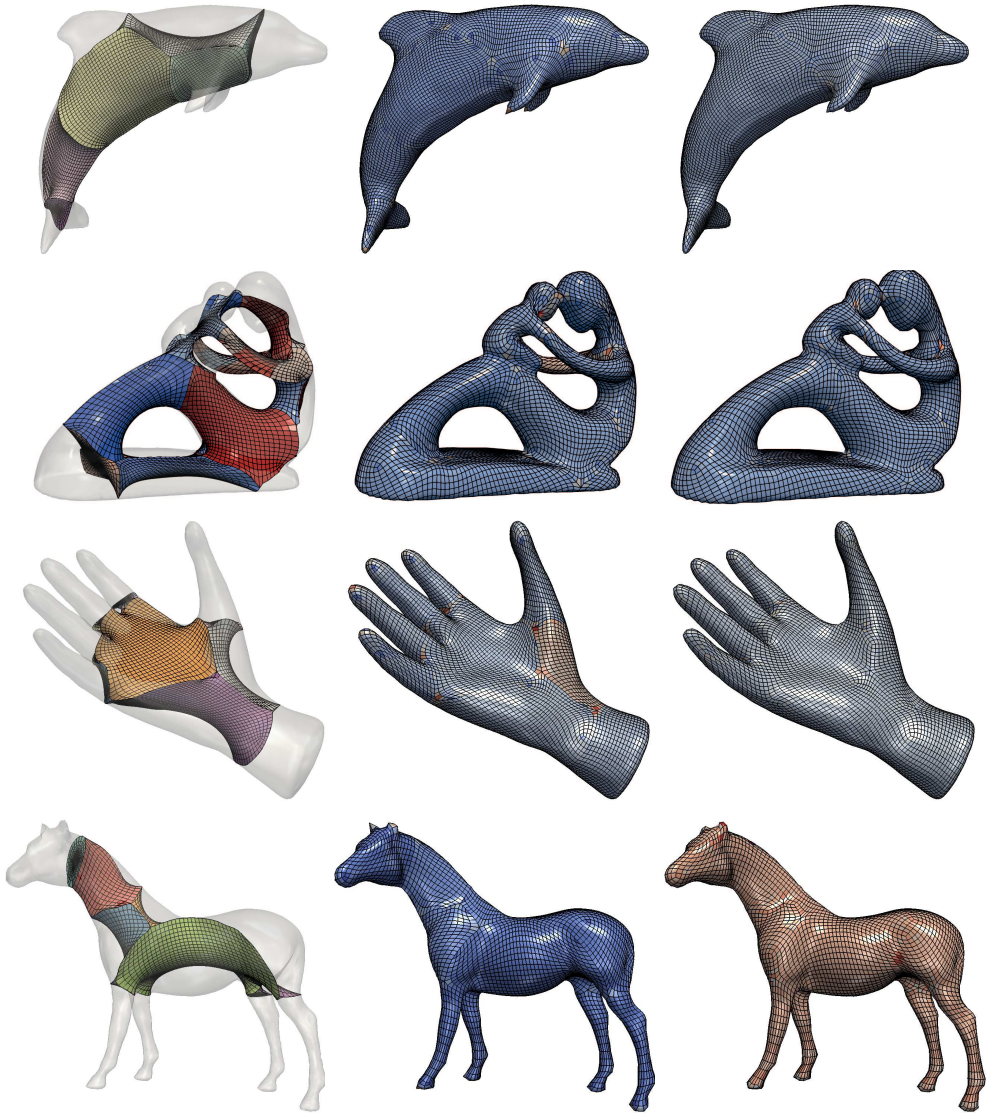
Figure 8. Example 1: Reconstruction results of different meshes. From left to right: input Basic Quad Layout S with the outline of M_\Delta in transparent, result of ALG_1 and result of ALG_2.
