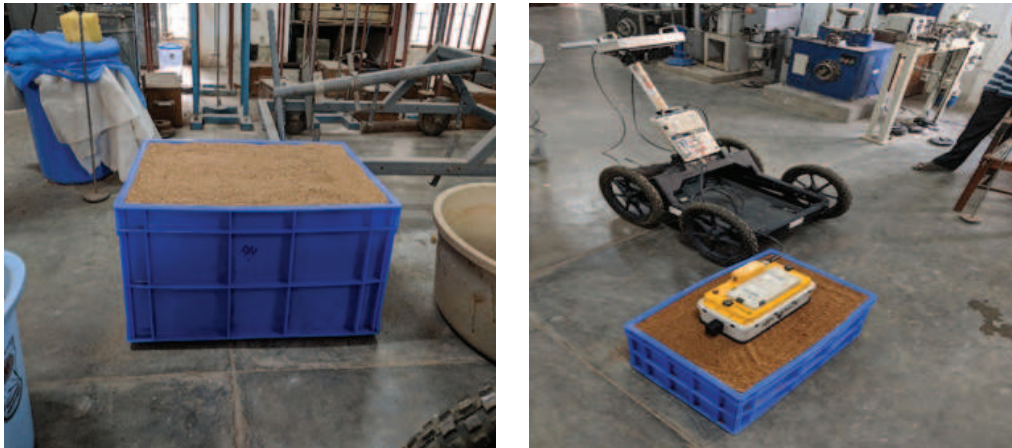
Figure 2: Picture of the soil plastic tank and GPR (Mala Inc., 800 MHz).
