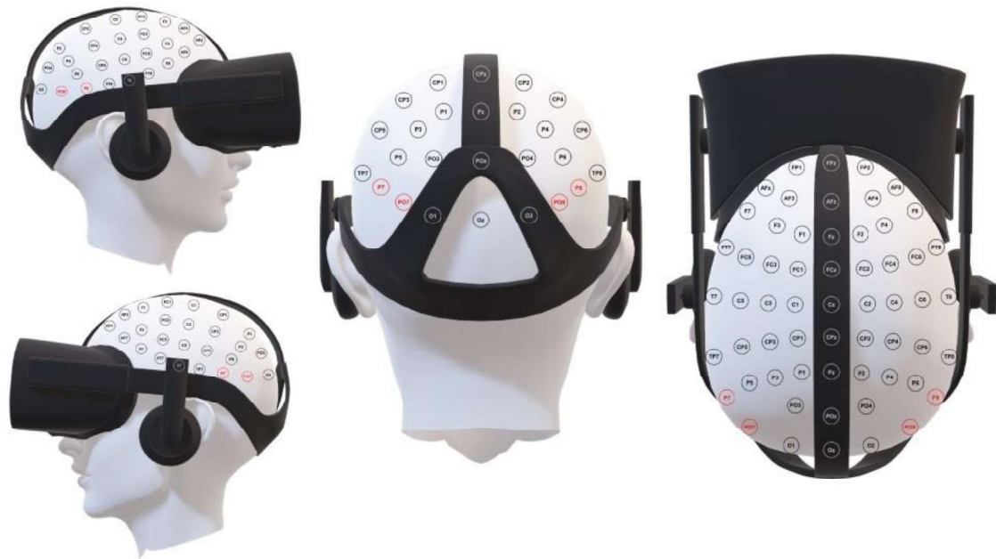
Figure 3. Illustration of the EEG/VR montage. As it can be seen in the illustration, the VR
