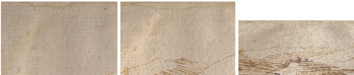
Figure 6: Paper shader RTR of the Landscape 1473 drawing with different light positions: zenithal (left), at 45° (center), raking (right).
