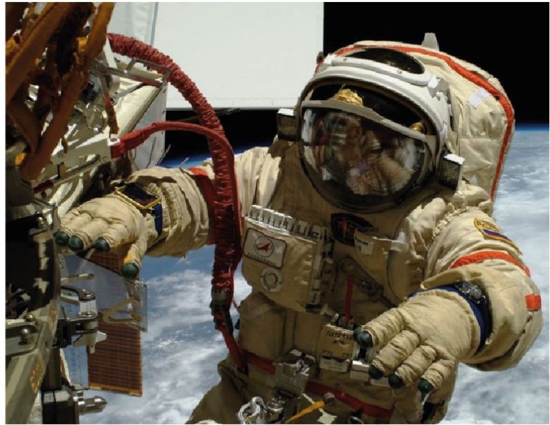
Fig. 2. Progression along a traverse with two safety tethers attached to a “ via ferrata ” handrail (left; photo Vittorio Crobu/ESA). This system shares several analogies with the tethers and protocols used during the Russian EVA techniques with the Russian Orlan spacesuit (right; photo credit NASA).
