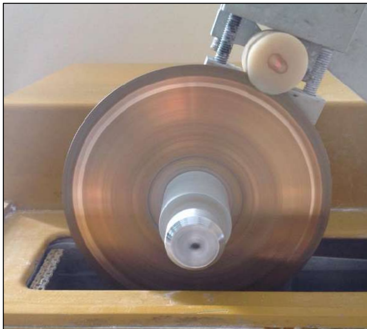
Fig. 8. Isomet diamond saw for the samples section cutting.
