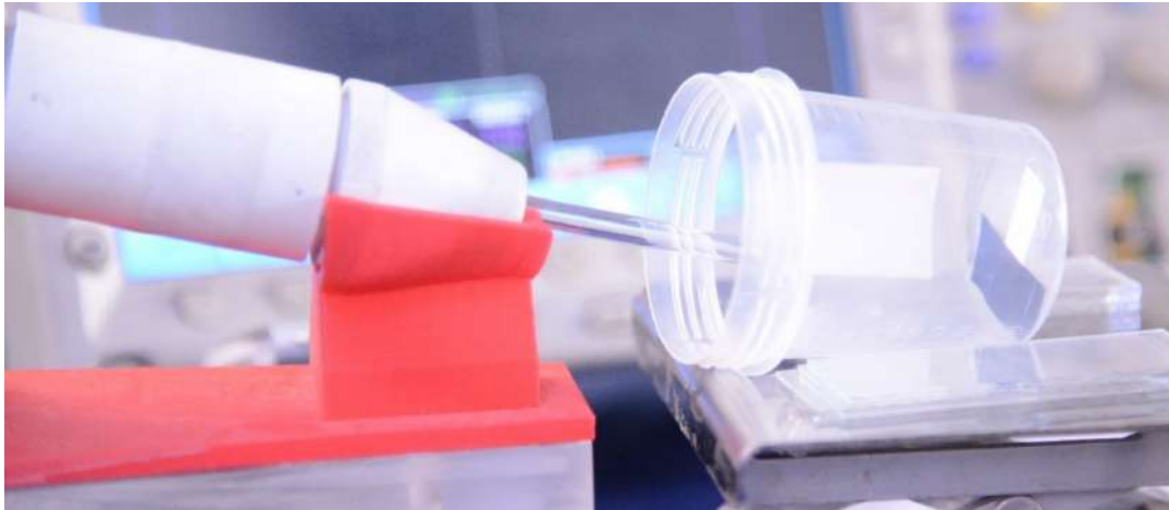
Fig. 3. Photo of ozone concentration measurement inside a chamber with one open boundary by means of ozone strips posed on the bottom of the chamber.
