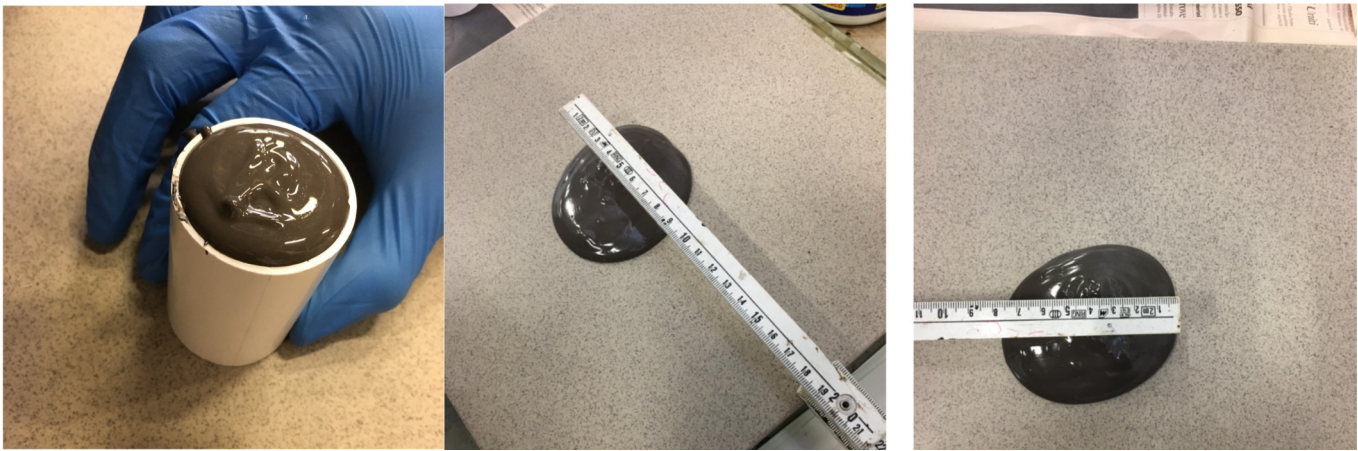
Figure 3. Fluidity testing for geopolymer mortars' fluidity.
