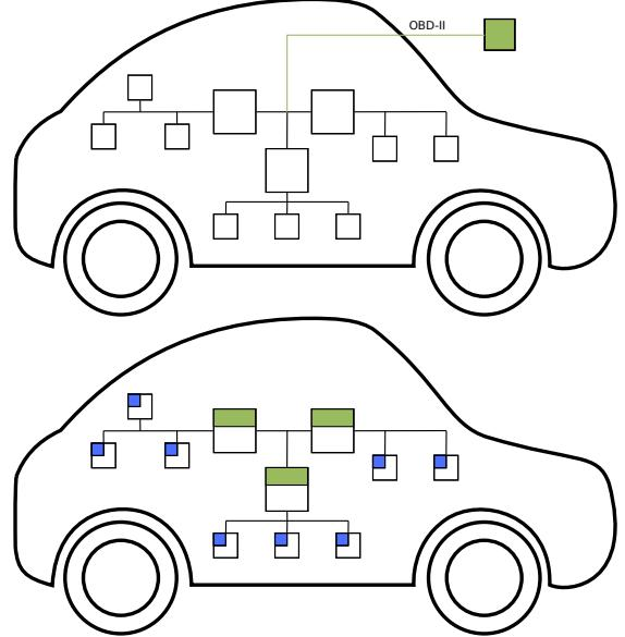
Fig. 3. *Safe-mode Manager* suggested topologies. Top: *External Independent SMManger*. Bottom: *Distributed Incorporated SMManger*. The *SMMangers* are marked in green, while the *SMClients* are marked in blue. Note that the upper figure shows one example for a system in *Transparent-mode*, while the lower one shows an example for a system in *Extended-mode*.
