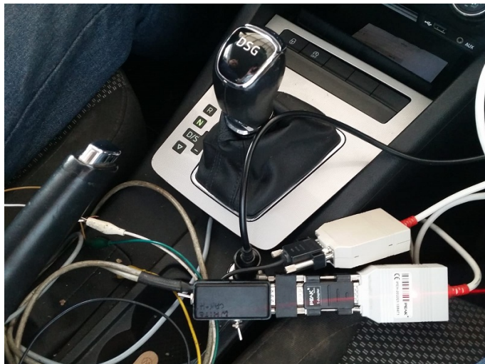
Fig. 5. CAN bus tapping. Note that both USB devices are connected to the same line by using the black T-connector.
