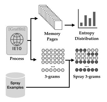
Fig. 1. Feature extraction overview. GLYPH extracts features for information entropy and memory byte n-grams from a process monitored by GRAFFITI.
