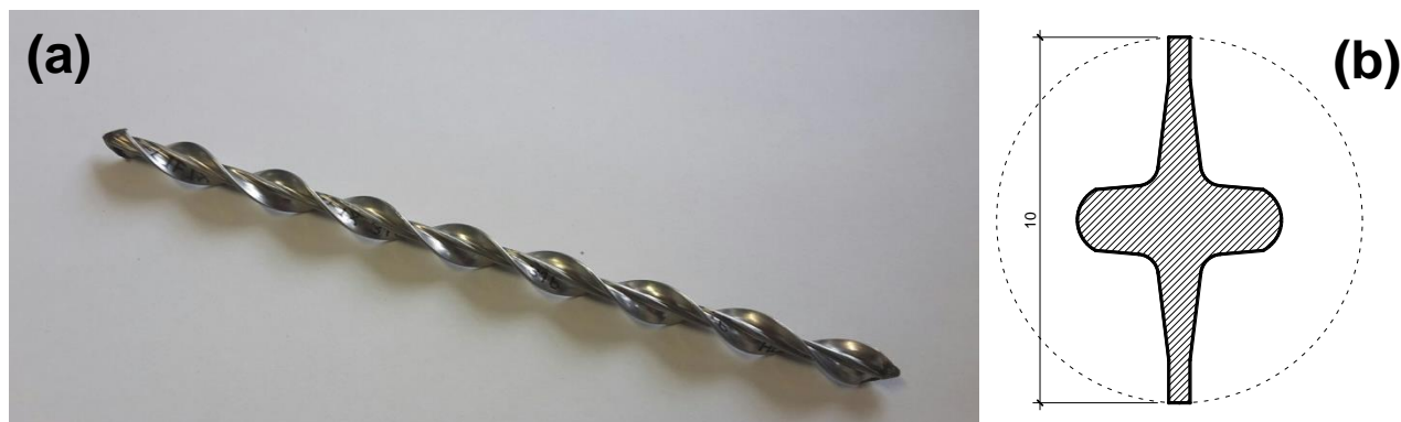
Fig. 1. a) Twisted bar and b) original cross-section of the bar before twisting (size in mm).
