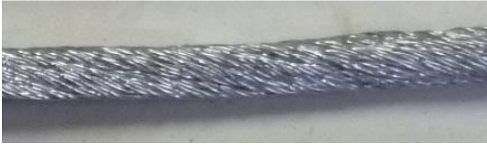
(c) CS conductor (short twist pitch)
