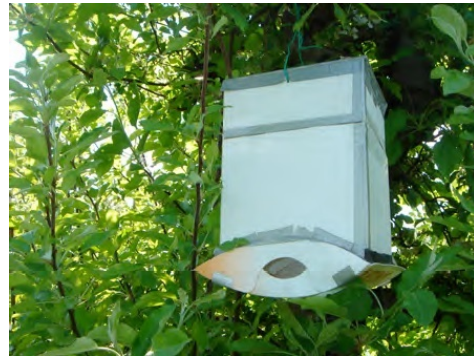
Fig. 1. Prototype of the IoT neural network Codling Moth smart trap.
