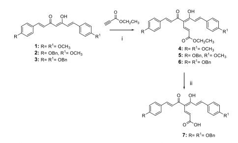
"Reagents and conditions: (i) NaH, dry THF, 0 °C to rt, N<sub>2</sub>, overnight, 41–84% yield; (ii) KOH (2 N CH<sub>3</sub>OH solution), CH<sub>3</sub>OH, 60 °C, 12 h, 75% yield.
