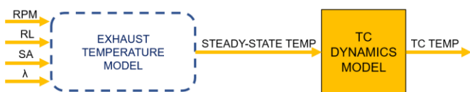
Figure 19. The exhaust manifold temperature model was coupled with the TC dynamic model in order to reproduce the TC signal also under transient conditions.
