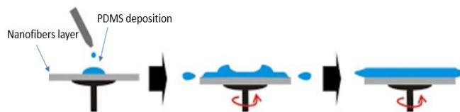
Fig. 4 Schematic principle of the spin coating process.
