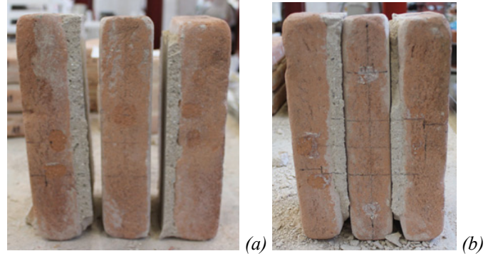
Figure 2. Typical failure modes of the triplet tests ( Type A ): (a) pure sliding along the brick-to-mortar interface; (b) sliding with mortar crushing at the joint extremities.
