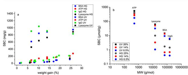
**Figure 7.** Equilibrium binding capacity of various target molecules onto heat and UV grafted ion exchange nonwovens: a) static binding capacity (SBC) in terms of mass adsorbed per mass of membrane as a function of % weight gain of polyGMA and b) static binding capacity on a molar basis as a function of the targets molecular weight for nonwovens grafted at 6.5%, 14%, and 25% weight gain.
