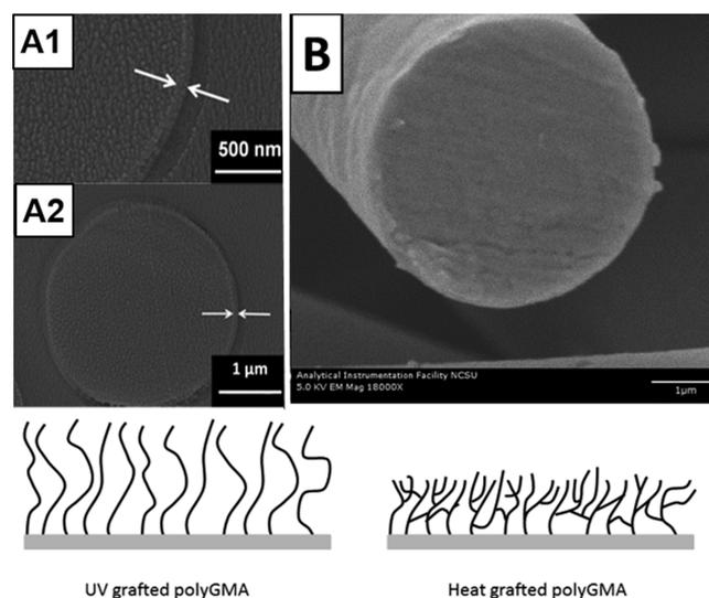
**Figure 6.** SEM images for PBT fiber cross sections grafted with A) UV (A1 and A2 are images with different magnifications of the same fiber)<sup>13</sup> and B) heat induced grafting. Schematic representation of polyGMA grafted layers resulting from UV and heat induced grafting.
