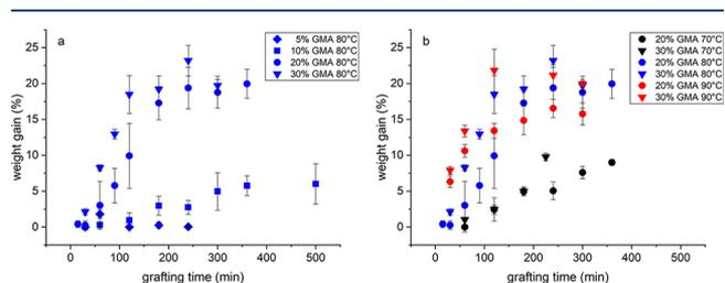
**Figure 2.** Heat induced grafting evaluated by % weight gain for a) different GMA concentrations (% v/v) at 80  $^\circ\text{C}$  and b) for 20 and 30% GMA at different polymerization temperatures over a range of polymerization times.
