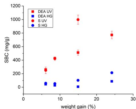
**Figure 5.** Equilibrium protein binding capacity of PBT nonwovens grafted by heat (30% (v/v) GMA, 80 °C) and UV light (20% (v/v) GMA) functionalized as anion (DEA) and cation (S) exchangers for capture of BSA and hIgG, respectively.
