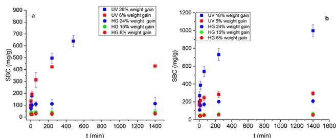
**Figure 8.** Static binding capacity at various contact times for ion exchange functionalized grafted nonwovens: a) BSA binding on anion exchange UV grafted at 20% and 6% weight gain, as well as heat grafted at 24%, 15%, and 6% weight gain and b) hIgG binding on cation exchange UV grafted at 18% and 5% weight gain, as well as heat grafted at 24%, 15%, and 6% weight gain.
