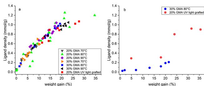
**Figure 4.** Ligand density of a) DEA and b)  $\text{Na}_2\text{SO}_3$  functionalized polyGMA grafted nonwovens.
