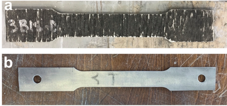
Figure 5: Tensile specimen cut from WAAM plates: (a) as-built and (b) machined.
