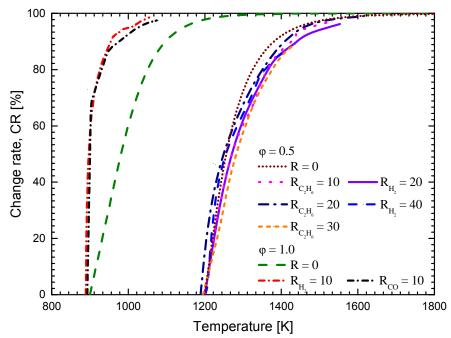
Figure 2: The effect of initial temperature on the changing rate (CR) of IDT for lean ( $\varphi = 0.5$ ) and stoichiometric ( $\varphi = 1.0$ ) compositions of premixed methane-air mixture added with hydrogen, ethane and carbon monoxide, as calculated by KiBo.
