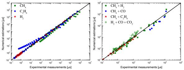
Figure 1: Comparison of ignition delay time data retrieved in the literature and estimated values for a wide range of conditions for pure methane, ethane, or hydrogen (left) and for bio-syngas representative mixtures (right).
