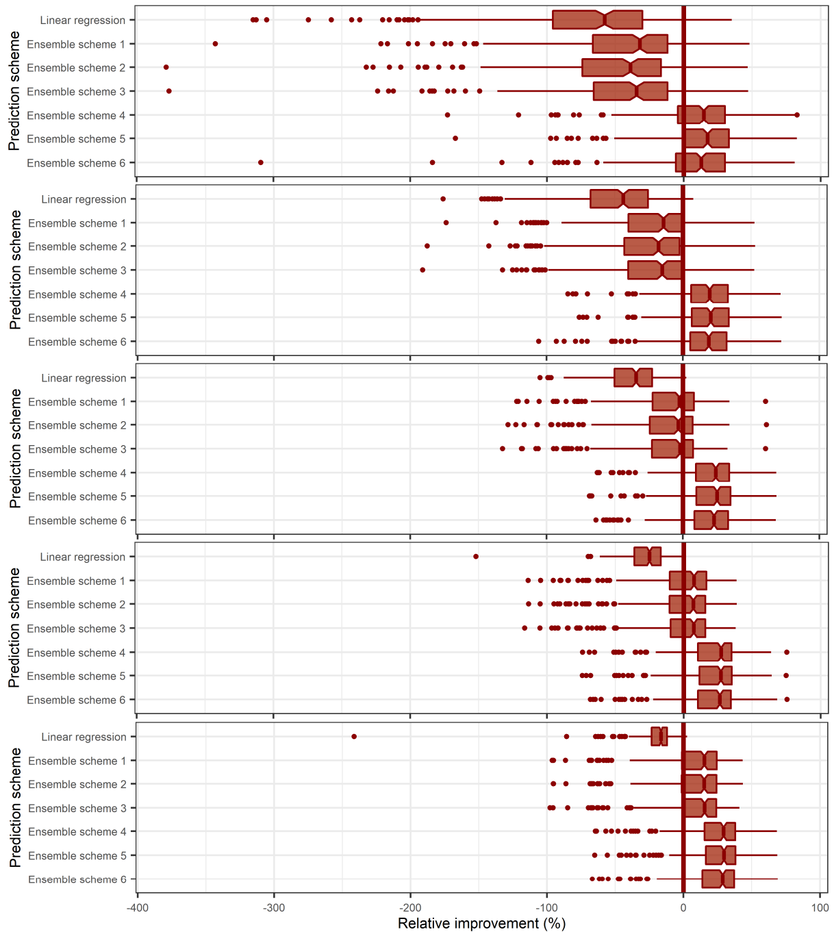
Figure 10. Relative improvements in terms of average interval score with respect to the quantile regression scheme for the 99%, 97.5%, 95%, 90% and 80% prediction intervals (from top to bottom) delivered by the compared schemes for the period T_3 (years 1975–1999). Each boxplot summarizes 270 values. The reference values (zero values) are denoted with red thick vertical lines.
