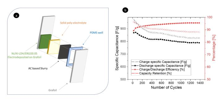
Figure 9: a) schematic representation of the hybrid SC; b) capacitance retention of the assembled SC at 2.5 A  $g^{-1}$  for 1,400 cycles
