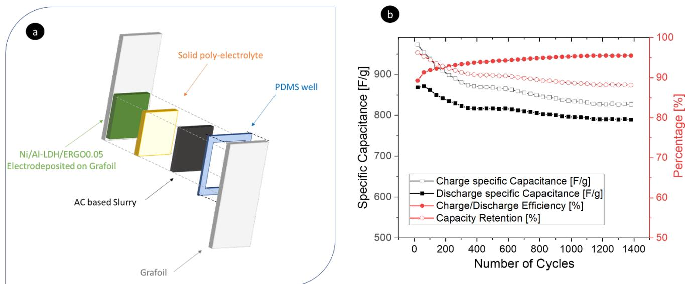
Figure 9: a) schematic representation of the hybrid SC; b) capacitance retention of the assembled SC at  $2.5 \text{ A g}^{-1}$  for 1,400 cycles
