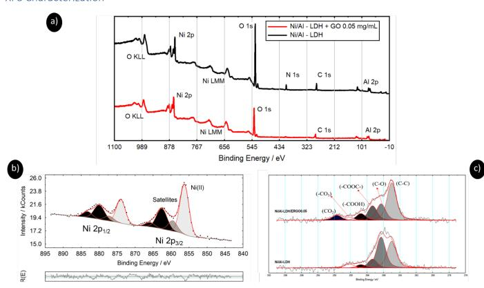
Figure 4: XPS data of a) normalized survey spectra of Ni/Al-LDH and Ni/Al-LDH/ERGO0.05 b) Ni 2p site of Ni/Al-LDH and c) comparison between C 1s of the pure LDH and LDH/ERGO0.05 composite (spectra have been normalized)
