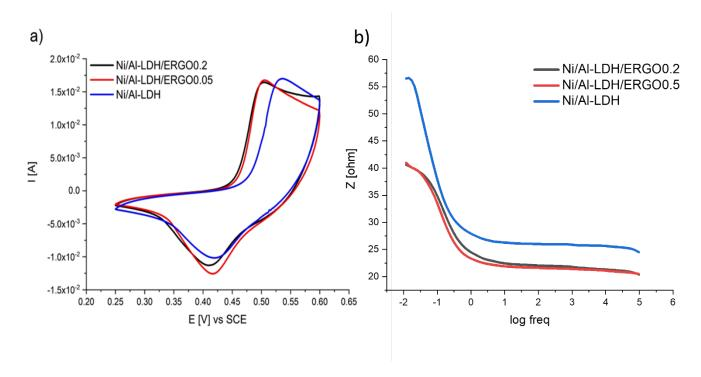
Figure 6: a) CVs of pure LDH and the composites Ni/Al-LDH/ERGO0.05 and Ni/Al-LDH/ERGO0.2 recorded at 10 mV/s; b)Bode plot for the same materials recorded when the applied potential corresponds to the maximum of the peak.
