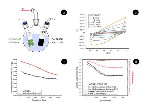
Figure 8: a) sketch of the set-up of the hybrid SC in solution; b) CVs at different scan rates of the asymmetric capacitor based of AC and Ni/Al-LDH/ERGO0.05 in 6 M KOH; c)comparison of the specific capacitance of Ni/Al-LDH and Ni/Al-LDH/ERGO0.05 during the continuous charge discharge cycling test at 2.5 A g<sup>-1</sup>; d) capacitance retention of Ni/Al-LDH/ERGO0.05 at 2.5 Ag<sup>-1</sup> for 20,000 cycles in solution.
