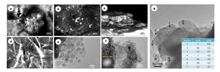
Figure 3: SEM images of a) Ni/Al-LDH b) Ni/Al-LDH/ ERGO1 c) cross-sectional view of Ni/Al-LDH/ ERGO0.2, and d) Ni/Al-LDH/ ERGO0.05. HREM-TEM images of e) Ni/Al-LDH, and f) Ni/Al-LDH/ ERGO0.05, inset: SAED pattern of ERGO g) TEM images of Ni/Al-LDH/ ERGO0.05; the open circles indicate the positions were the EDS spectra were collected. In the table the ratios between  $C_k/Al_k$  and  $C_k/Ni_k$  counts are shown.
