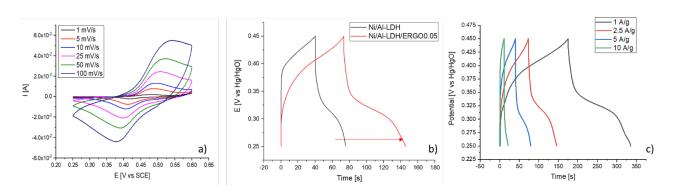
Figure 7: a) CVs at different scan rates of Ni/Al-LDH/ERGO0.05 in 0.1 M KOH; b) comparison of GC-D curves of Ni/Al-LDH/ERGO0.05 and Ni/Al-LDH at 2.5 A  $g^{-1}c$ ) GC-D curves recorded at different current densities for Ni/Al-LDH/ERGO0.05.
