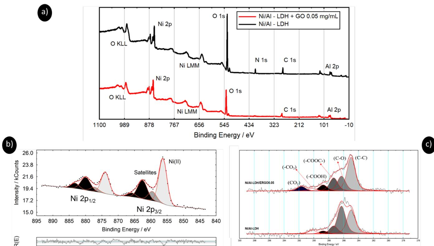
Figure 4: XPS data of a) normalized survey spectra of Ni/Al-LDH and Ni/Al-LDH/ERGO0.05 b)  $2p$  site of Ni/Al-LDH and c) comparison between  $C 1s$  of the pure LDH and LDH/ERGO0.05 composite (spectra have been normalized)
