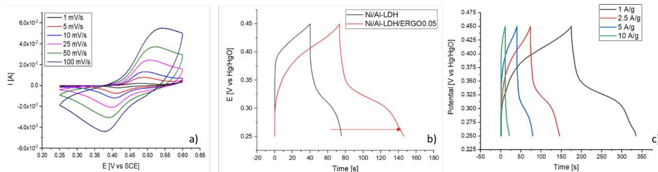
Figure 7: a) CVs at different scan rates of Ni/Al-LDH/ERGO0.05 in 0.1 M KOH; b) comparison of GC-D curves of Ni/Al-LDH/ERGO0.05 and Ni/Al-LDH at 2.5 A g<sup>-1</sup> c) GC-D curves recorded at different current densities for Ni/Al-LDH/ERGO0.05.
